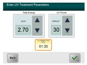
Figure 3-8. Pulsed UV Treatment Parameters Screen
