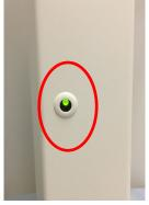
Figure 3-31. KXL System Battery Status Indicator
