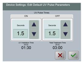
Figure 3-39. Edit Default UV Pulse Parameters (Pulsed Only)
