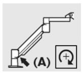
Figure 4-4. With Arm Raised, Tighten Set Screw (A)
