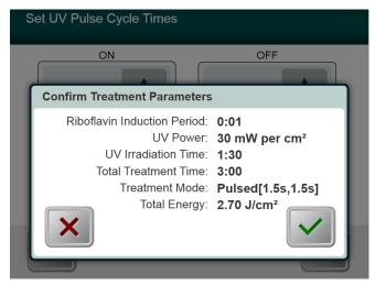
Figure 3-10. Confirm Pulsed UV Treatment Parameters Screen
