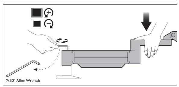
Figure 4-3. Turn the Adjustment Screw
